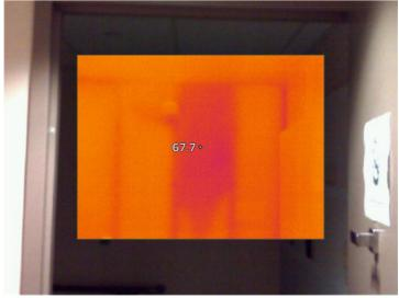
IR000138.IS2 5/4/2011 10:57:45 AM Poorly installed insulation in one wall cavity
