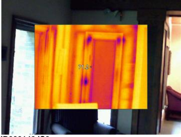
IR000142.IS2 5/4/2011 11:06:44 AM Shows typical air infiltration around window trim
