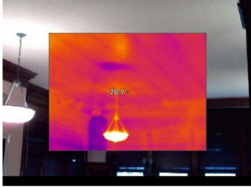
**IR000114.IS2** 5/4/2011 9:49:37 AM Section of missing insulation in ceiling. A similar area was also seen on the other side of the room
