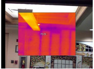
**IR000103.IS2** 5/4/2011 9:25:56 AM Missing or settled insulation at the top of wall cavities
