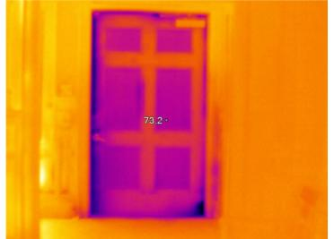
**IR000126.IS2** 5/4/2011 10:37:20 AM Air infiltration around edge of door. Daylight can be seen through gaps at several places.
