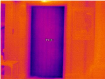
**IR000135.IS2** 5/4/2011 10:52:45 AM Significant air leage is coming from elevator shaft
